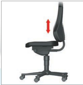
Backrest height and seat tilt adjustment
